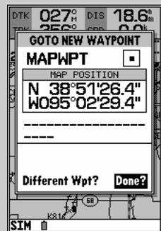
If no waypoint is highlighted at the cursor position, you can still go to the position. The GPSMAP 195 automatically creates a waypoint named 'MAP-WPT'.
