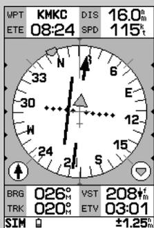
Use the **⦿** keypad to 'drive' simulator mode operations. The UP/DOWN arrows control speed. The RIGHT/LEFT arrows control ground track.
