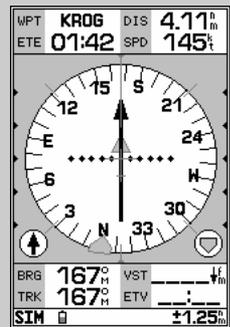
Once you are within 500 feet of the target altitude, the 'Approaching Target' message will appear, and the VNAV indicator will be removed from the HSI display.
