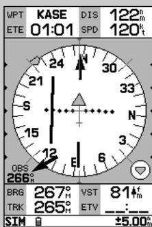
The 'Set OBS and Hold?' function allows you to specify an inbound heading to a destination waypoint. When this option is selected, an OBS heading appears in the bottom left corner of the HSI display. Use the
