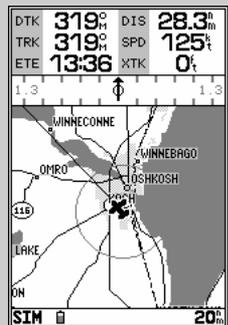
The compass may be replaced with a graphic CDI, to provide course guidance on the map page. You can also add additional data fields to the display (six in this example).
