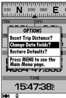
The GPSMAP 195's position page features a context-sensitive options page providing access to settings and special features of the position page.
