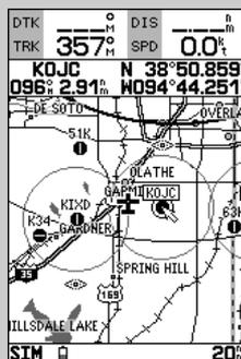
To select an on-screen airport, nav aid or waypoint; simply move the cursor over the desired waypoint. The name and position, along with the bearing and distance to that point, from present position, will appear:
