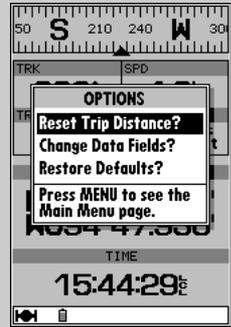
To reset the trip (TRP) odometer, select 'Reset Trip Distance?' from the position page options.
