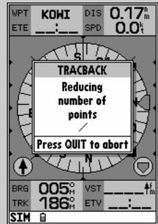
To stop the TracBack function before a route is created, press the **QUIT** key while the progress window is displayed.
