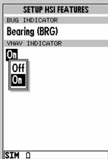
To turn the VNAV indicator on or off, select 'Setup HSI Features?' from the HSI options page. By default, the VNAV indicator is turned on.
