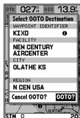
On many screens that display a waypoint name, or a list of waypoint names, you can highlight the waypoint name before pressing the key. This allows you to quickly select a GOTO destination without having to enter the name. You may find this a very useful timesaving tool. (You may recall from the nearest waypoints section that this method was used to select a nearest airport and go to that airport.)
