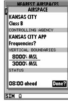
When an airspace alert message is provided, the **NRST** key can provide additional detail about the airspace. The nearest airspace page lists the six nearest airspaces for which airspace alerts have been issued. Normally, only one or two airspace alerts will occur at a time, but with sectorized controlled-airspace (such as many Class B areas) you can have more.
