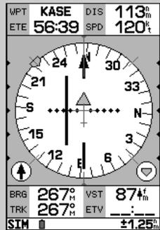
*This example shows the aircraft heading parallel to the desired course, to the right more than 0.5 nm.*
