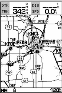
During normal use the GPSMAP 195 will automatically sequence to the map page once enough satellites are received to compute a position fix.
