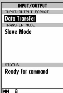
The 'Data Transfer' option allows the GPSMAP 195 to exchange track log, waypoint, almanac, and route data with a personal computer or another GPSMAP 195.
