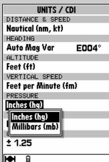
Barometric pressure figures may be entered/displayed in inches of mercury or millibars.
