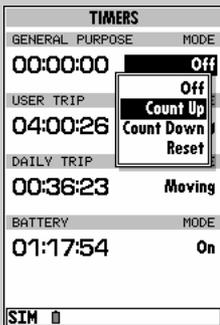
The general purpose timer field offers a count up and count down timer. You may also select from a variety of other timers to keep track of trip times, battery life or elapsed time using the other timer options.
