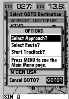
'Select Approach?' allows you to replace the GOTO destination airport with the final course waypoints of a published approach. This option is also used to select a different approach to the same airport.
