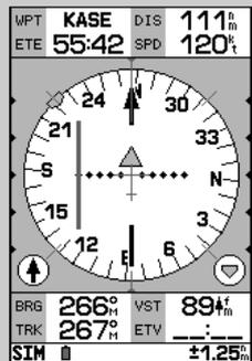
*This example shows the aircraft even further off course beyond the limits of the CDI scale. The D-bar will stay at the edge of the scale until your cross-track error is less than the limits of the scale.*
