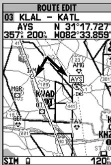
New waypoints can be added to an existing route by using a “rubber band”. Point to the route leg you wish to add to and press **EDIT**. Drag the “rubber band” to the new waypoint and press **EDIT**.
